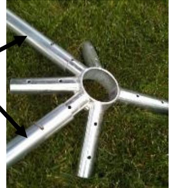
\*Connect the 14'4" hip rafters (red) to the 6 way crowns by placing the R pin in the alignment hole. The alignment hole is closest to the center of the 6 way crown. Slide the tube on the extension. The R pin alignment hole prevents the tube from sliding too far onto the extension.
